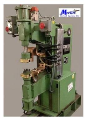
Schlatter P1 40kVA spot/projection welder, overhauled, modern weld control unit, adjustable lower welding electrode height.
